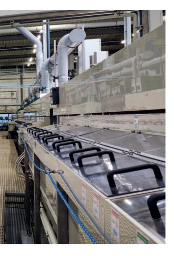
Electroplating stands as a cornerstone in modern manufacturing, offering a multitude of benefits including improved corrosion resistance and increased durability. This process involves the deposition of a metal coating onto a conductive substrate through the application of an electric current.
